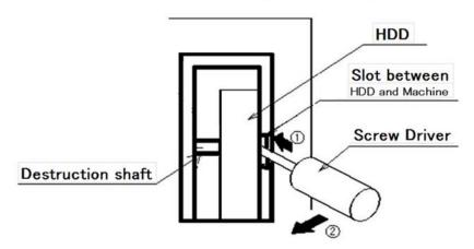
If you insert the HDD incorrectly, the Destruction Shafts may be damaged Refer to the manual for further information.
